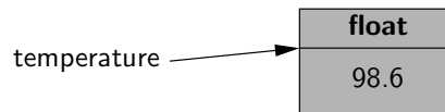
Figure 1.1: The identifier temperature references an instance of the float class having value 98.6.
