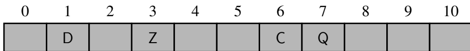
Figure 10.3: A lookup table with length 11 for a map containing items (1,D), (3,Z), (6,C), and (7,Q).
